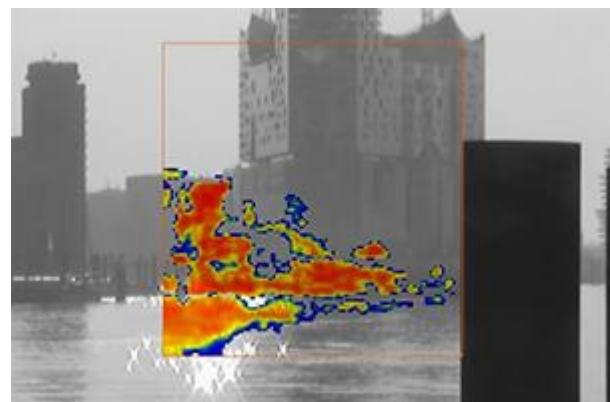
Measurement of ethylene and ammonia ( $\text{NH}_3$ ) emissions from different sources on an industrial area:
